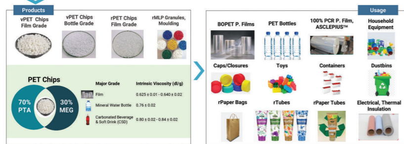
1. Mono ethylene glycol (MEG); 2. Purified terephthalic acid (PTA); 3. post-consumer recycled (PCR); 4. Polyethylene terephthalate (PET); 5. Virgin polyethylene terephthalate (vPET); 6. Recycled polyethylene terephthalate (rPET); 7. recycled multi-layered and multi-layered plastic packaging (MLP); 8. Biaxially oriented polyethylene terephthalate(BOPET); PET Production RM: 70% PTA, 30% MEG by Weight; sciencedirect.com
